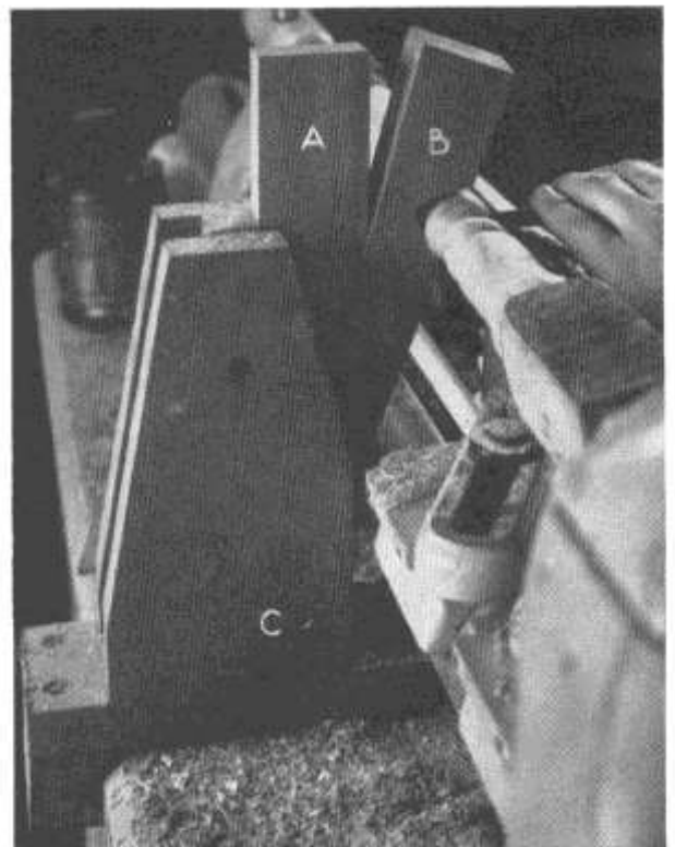
FIG. 8. SIMPLE WOOD STEADY MADE FOR MYFORD LATHE. The idea could be adapted to suit any make of lathe. (A) is the wedge which tends to drop down by gravity and keep the slip (B) up to the work. The slip is pivoted at C).
