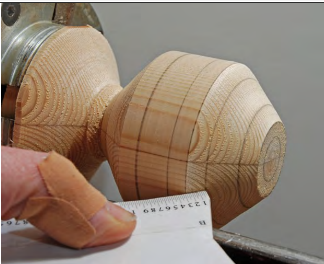
Fig04: Measuring from each corner of the octagon with the smaller scale.
