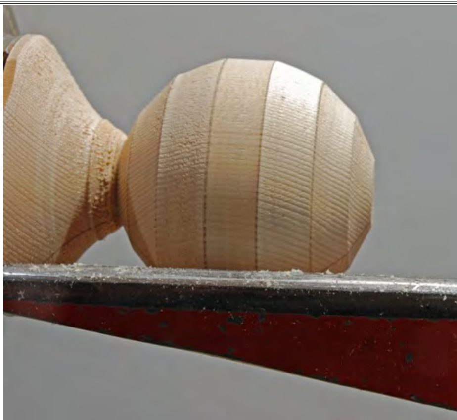
Fig05: After cutting away the corners of the octagon between the lines.
