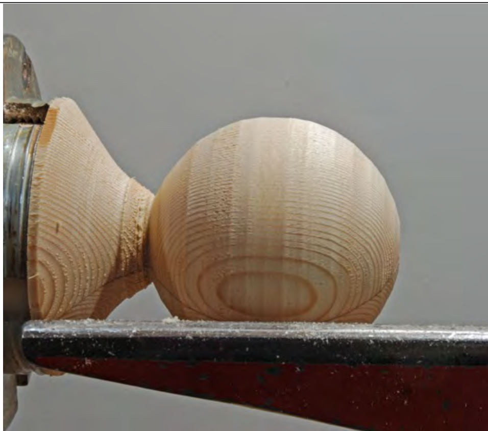
Fig06: After rounding over the corners of the hexadecagon.
