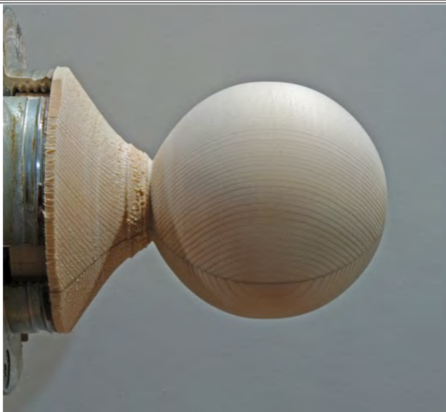
Fig07: After the final shaping with abrasives.
