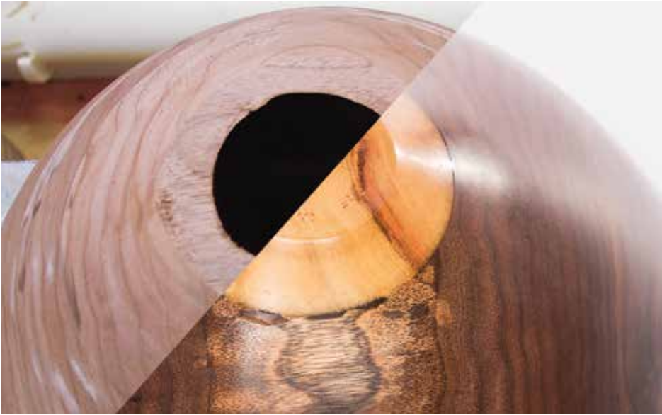
Before and after. If you have misjudged the bottom thickness of a bowl and turned through it, consider a contrasting plug to save the day.
