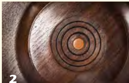
Decorative grooves were turned on the foot surrounding the plug to help integrate it visually.
