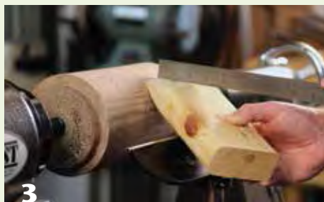
3 Skewing the angle of the tool effectively produces a “sharper” edge, which generates a shearing or paring action and ultimately a cleaner cut surface.
