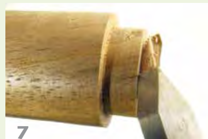
To achieve a clean cut on endgrain, use just the toe of the skew chisel. To avoid a catch, lean the left-side bevel slightly away from the endgrain (exaggerated here to illustrate the concept).
