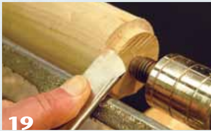
19 The peeling cut is made with the skew held flat on the toolrest. The 90° angle between the cutting edge and the toe of the skew is important to make this cut successful.
