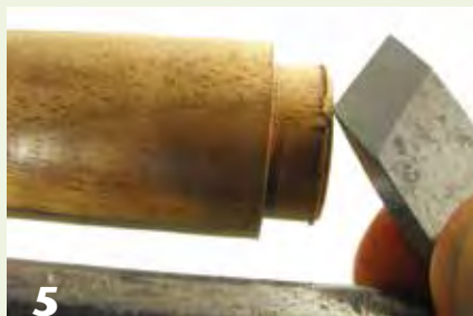
Position the bevel of the skew chisel parallel to the wood to begin cutting a fillet.
