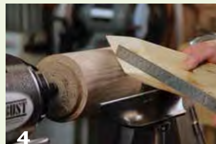
3 Skewing the angle of the tool effectively produces a “sharper” edge, which generates a shearing or paring action and ultimately a cleaner cut surface.
