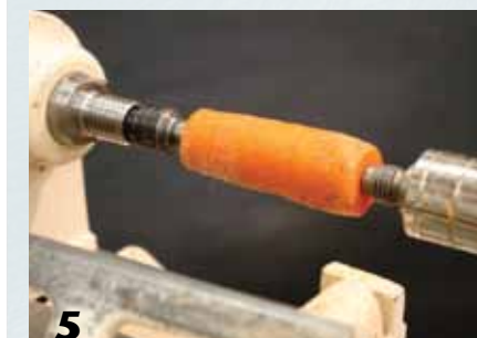
5 Cut a large carrot to about 4" (10 cm) long and mount it between centers.
