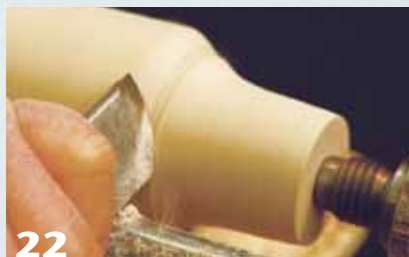
22 To learn how to make a cove cut, practice first on the end of a piece of wood. Next try turning a complete cove in the center of the cylinder by cutting from both ends and meeting at the middle. Most likely, you will find that coves, especially smaller ones, are a lot easier to make using a spindle gouge.
