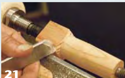
21 The pommel cut is also like a V-groove cut and is used for making a transition from square to round.
