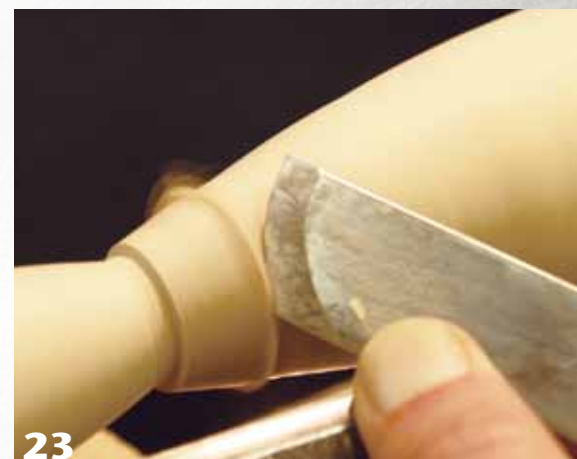
23 Practice your new skills by turning a candleholder with the skew chisel.
