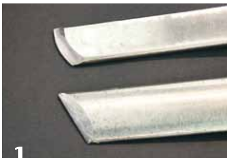
1 My favorite skew chisels: a 1¼"- (3 cm-) wide rectangular skew with a curved cutting edge and a concave bevel (top) and a 1½"- (4 cm-) wide oval skew with a straight edge and flat bevel.
