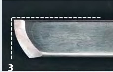
3 The edge at the toe of the curved skew is at 90° to the top of the tool, and has a short (no more than \frac{1}{4} " [6 mm]) straight section before starting the curve.
