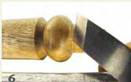
Finish cutting the fillet by advancing the tool as you would for a planing cut.
