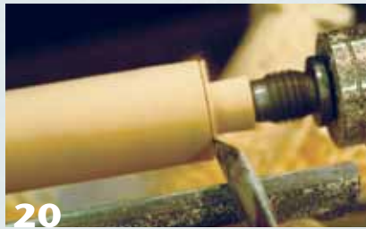
20 The facing cut is made like the V-groove cut except that the result is a 90° shoulder on the wood. Make sure there is a slight clearance between the wood and the side bevel of the skew.
