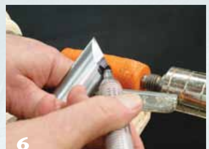
6 Mark the lower half of the bevel with a permanent marker. This will identify the safety zone.
