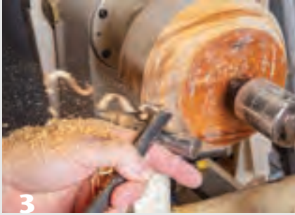
Rough-shaping the mortar's outside profile, cutting toward the headstock and across the facegrain. The blank is mounted between centers.
