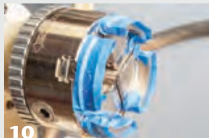
Painter's tape protects the wood as you gently expand the jaws inside the mortar rim for a good grip. Use the tailstock live center to aid in centering.
