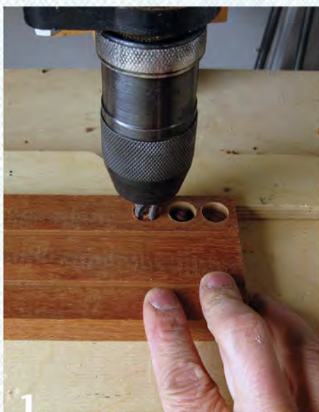
Chuck a \frac{1}{4} " plug cutter in the drill press to make plugs of a contrasting wood.
