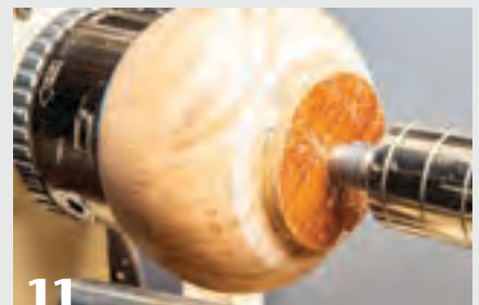
Painter's tape protects the wood as you gently expand the jaws inside the mortar rim for a good grip. Use the tailstock live center to aid in centering.
