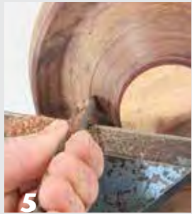
4 The author's deep-fluted "trimmer" gouge, used for making smooth finishing cuts on both the outside and inside of bowls.
