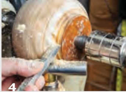
Beginning to form a tenon at the tailstock end of the blank.
