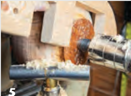
The author's tenon-sizing gauge, made from scrap wood, used to quickly form a tenon you know will fit in your chuck.
