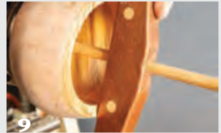
Deepen to desired bottom thickness, checking often with a depth gauge.
