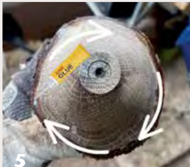
5 The author applies CA glue around the bark to increase the chances of it staying intact.
