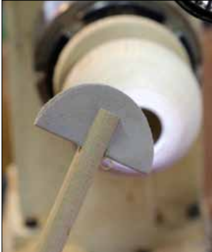
24 Sanding aid. To sand the inside, fold a disk of sandpaper into the slot in a dowel.
