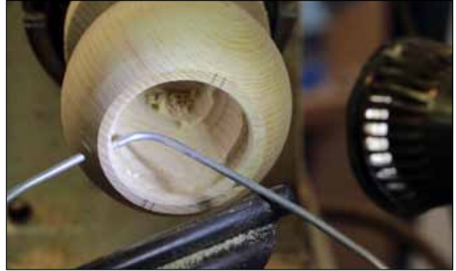
22 Wall thickness. Move the caliper along the inside wall and eyeball the gap on the outside.
