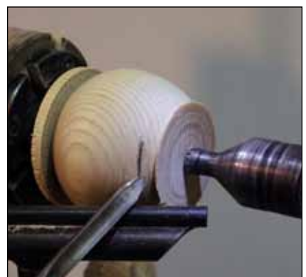
29 Remount. Plug the hollow form onto the jam chuck and bring up the tailstock live center.
