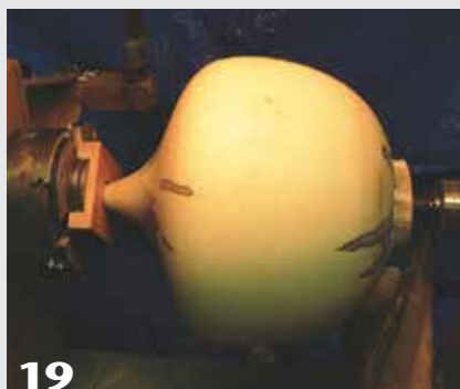
18 A shopmade O-ring jam chuck allows the author to remount the piece to complete the bottom. The spout fits into the jam chuck hole, and the tailstock holds it in place.
