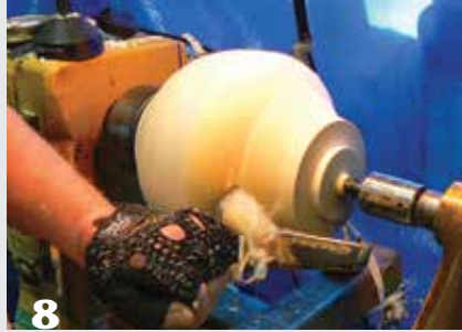
8 With the tailstock brought up for added support, continue shaping the hollowform.
