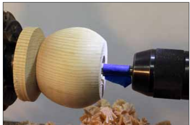
15 Bore. Mount the drill bit in a tailstock chuck and bore in stages to the exact bottom depth.
