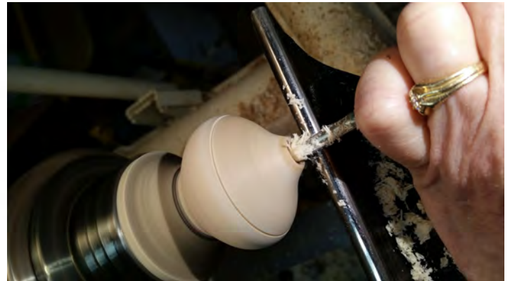
Photo 2. Using the spindle gouge to widen the initial pilot hole.
