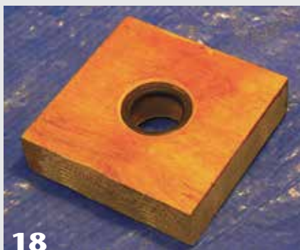
18 A shopmade O-ring jam chuck allows the author to remount the piece to complete the bottom. The spout fits into the jam chuck hole, and the tailstock holds it in place.
