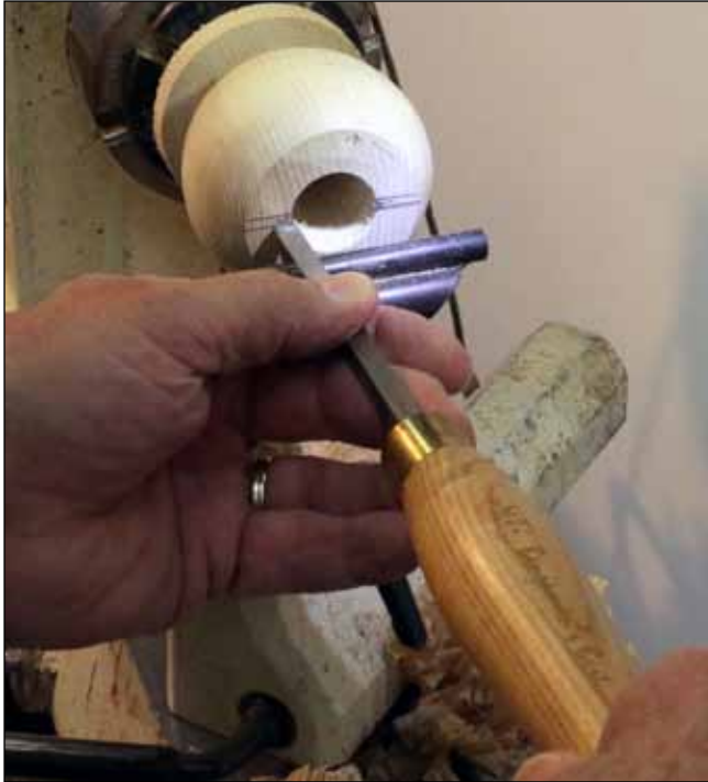
16 Scraper setup. Set the toolrest so the straight hollowing tool cuts on center with its handle horizontal and parallel to the lathe axis.
