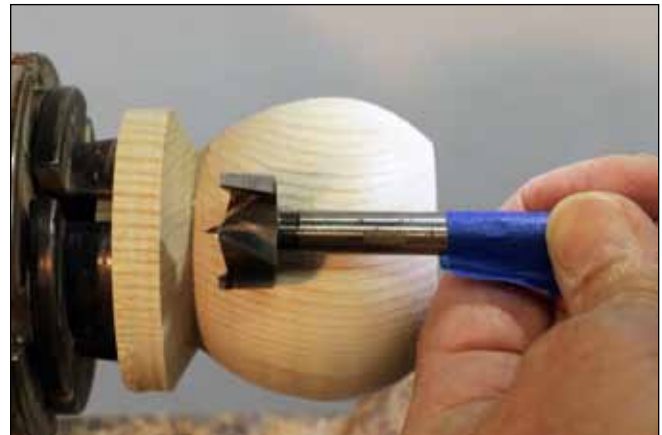
14 Depth gauge. Mark the depth with tape so the point of the bit indicates the pot's bottom inside.
