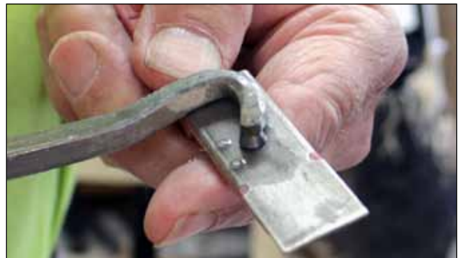
6 Hone carbide. Hone across the flat surface with a drop of water or light oil.
