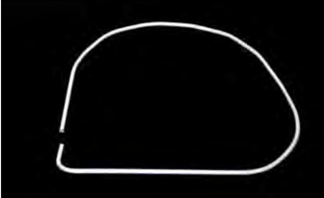
21 Caliper. A loop of coat-hanger wire, or #14 iron wire, can be bent into a wall-thickness gauge.
