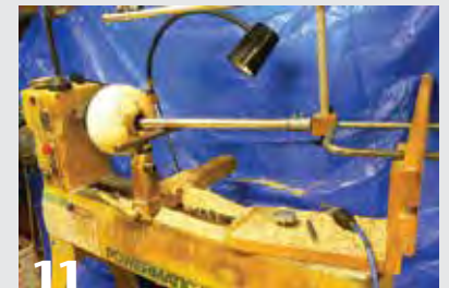
11 The author's hollowing rig, a captured boring bar system.
