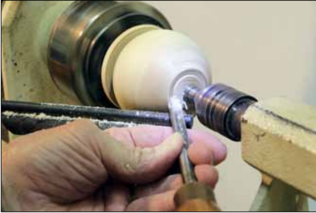
30 Cut the foot. Undercut the bottom so the form has a foot that sits flat on the table.
