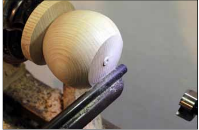
13 Remount. Grip the tenon in a scroll chuck, face off the end, and make a drill-centering divot.
