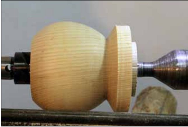
12 Outside shape. Shape the outside of the pot, leaving wood for a foot on the tenon side.
