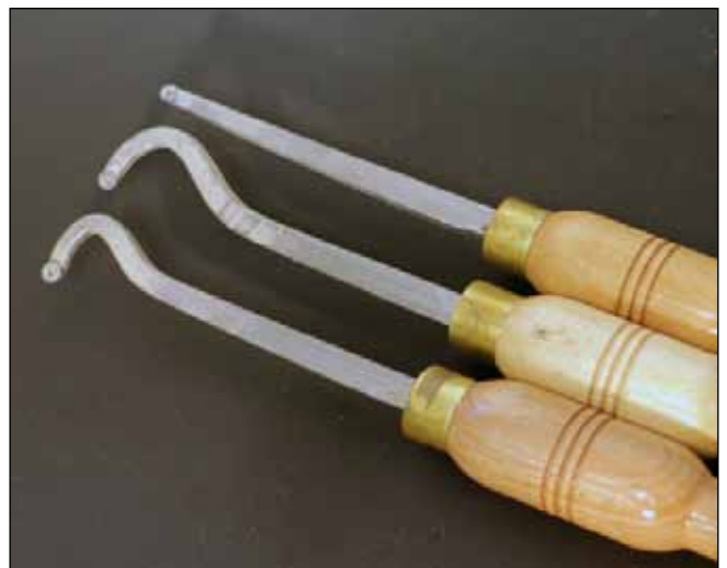
2, 3 Tools. All hollowing tools are scrapers, with straight and bent shanks to reach everywhere inside a vessel. Steel tools, top, and carbide-tipped tools, right.
