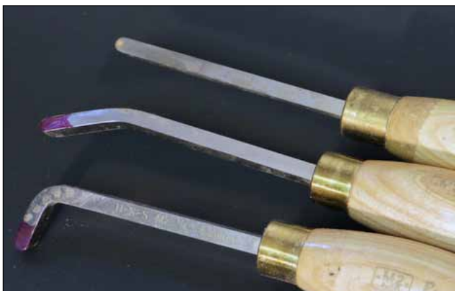
2, 3 Tools. All hollowing tools are scrapers, with straight and bent shanks to reach everywhere inside a vessel. Steel tools, top, and carbide-tipped tools, right.
