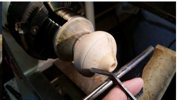
Photo 5. 45° hollowing tool, made from an allen wrench.
