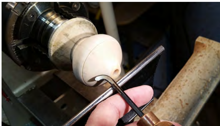
Photo 4. 90° hollowing tool, made from an allen wrench.
