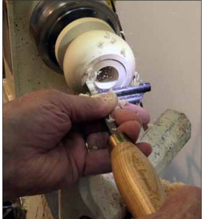
17 Cutting. Take shallow cuts by sliding the tool along the rest from the center opening toward the outside.
