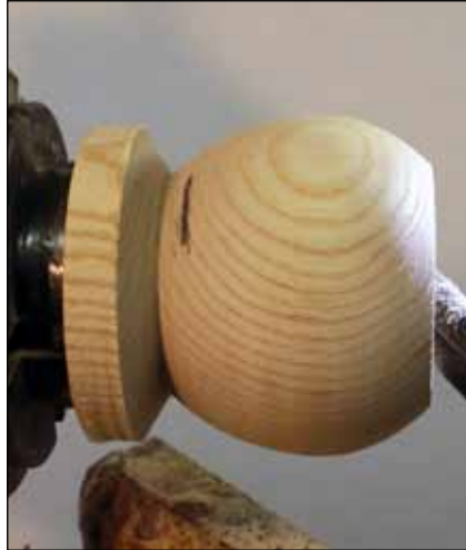
25 Mark bottom. Measure and mark the inside bottom on the outside of the form.
