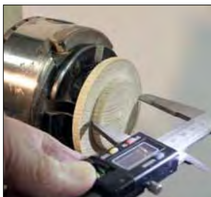
28 Jam chuck. Cut a tenon on the waste block, sized to fit the opening.
