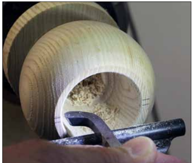
18 Walls. Establish uniform wall thickness near the opening before hollowing to full depth, using the bent tools.
