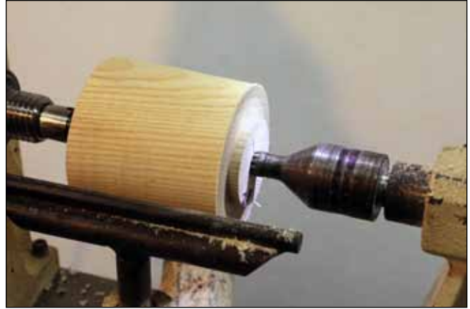
8 Tenon. Rough-turn to a cylinder with a chucking tenon on one end.
