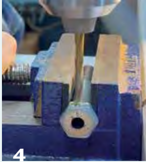
The author drills a hole and then taps threads for the cap screw, which will hold the blade in place during use.
