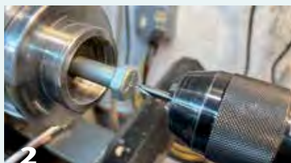
Use a center drill to create a dimple, or starting point for the drill bit.
