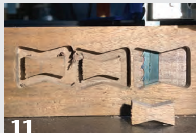
Once several butterfly inserts have been routed, remove them from the parent wood using a bandsaw or table saw with a zero-clearance insert.
