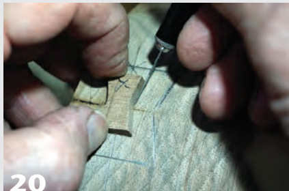
20 Use a sharp knife to scribe a fine line on the bowl, indicating how much material to remove from the sides of the recess for a good fit.
