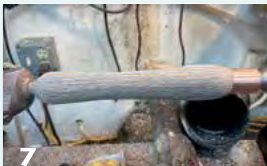
Turn a handle with a ferrule. A hole drilled into the end will accept the bolt, or rod.
