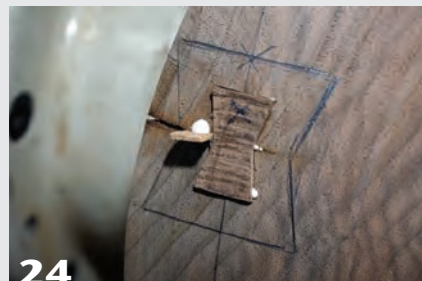
24 A wood wedge, or splinter, is used as a dam to prevent glue from squeezing into the crack.
