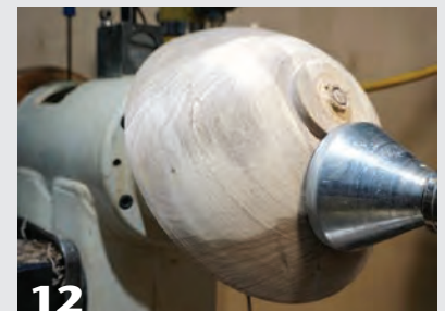
Mount the bowl (on or off the lathe) in such a way that the cracked work area is horizontal.
