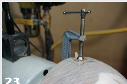
23 With glue applied, set the inlay into the recess. If the patch is near the bowl rim, a clamp will do the job; if not, gently tap in the inlay.
