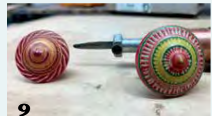
The author presents the side of the flexible blade to the hardwood endgrain, producing intermittent cuts. Adding color accentuates the chatter marks beautifully.
