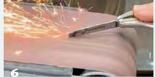
A jigsaw blade will serve as the chatter tool cutter. Grind off its teeth and shape it using a grinder or belt sander.
