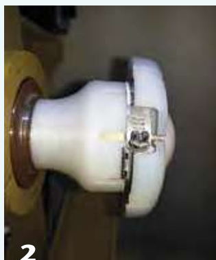
A hose clamp enclosed in a shroud is used to tighten this 3D-printed collet chuck.
