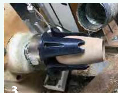
Chuck jaws can be printed to any specified design, here customized for a small vase.
