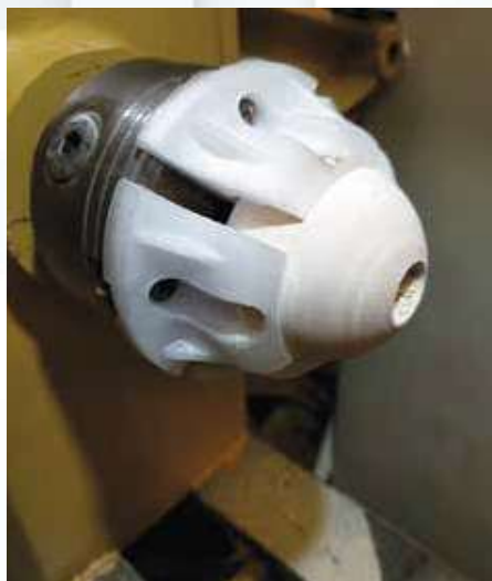
Custom 3D-printed soft jaws hold a sphere for turning.
