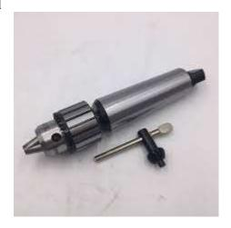
For severe applications, you will notice a tang on the end of the taper that is designed to engage in a slot to prevent the taper from turning under load. In milling machine applications, a draw bar is used to pull and hold the taper into the socket. This is important, because with cyclic sideways loading from a cutter as it turns and cuts, the taper can actually work loose, because there is no axial loading to keep the taper in the socket.
