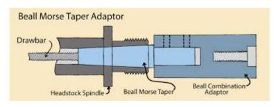
socket to ensure that the taper locates properly and does not spin in the socket. If it does spin, it is likely to pick up burrs and damage the socket, ruining the accuracy of the machine. Tools such as drive centres are relatively easy and cheap to replace. However the socket usually forms part of the lathe spindle or the tailstock and is expensive to replace, so it is important to avoid damage, such as may be caused by the taper spinning in the socket.
