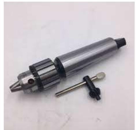
For severe applications, you will notice a tang on the end of the taper that is designed to engage in a slot to prevent the taper from turning under load. In milling machine applications, a draw bar is used to pull and hold the taper into the socket. This is important, because with cyclic sideways loading from a cutter as it turns and cuts, the taper can actually work loose, because there is no axial loading to keep the taper in the socket.
