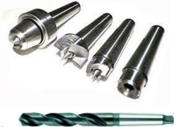
There are a number of standard tapers used in machines. In the woodturning world, Morse Tapers are almost universally used. Morse tapers are one of a class of “self-holding” tapers. The means it is a narrow angle taper (about 1.5°) designed to hold in the socket by friction alone and will not easily fall out. There are other standard tapers used in other applications such as milling machines.
