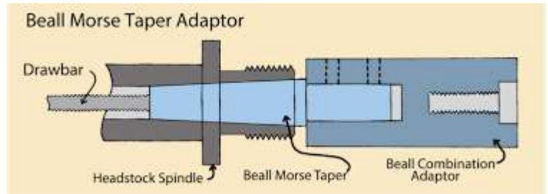
When installing a tool with a taper into a socket, it is important to remove any dust or swarf from the taper and the
