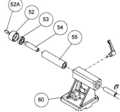
significant radial and axial loads and should last a lifetime. If you look at the data sheets and the bearing life calculator provided by the manufacturer, you will see that even at the highest speeds the Jet Mini can run at, with the largest work-pieces and high tail stock pressures, the life is given in thousands of hours. But the live centre supplied with my lathe failed.
